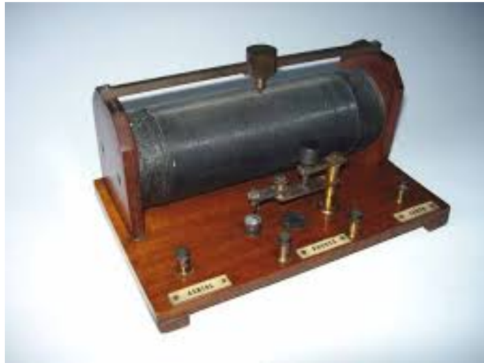
Figure 3 - Crystal receiver (note galena crystal and “catwhisker” in middle)
